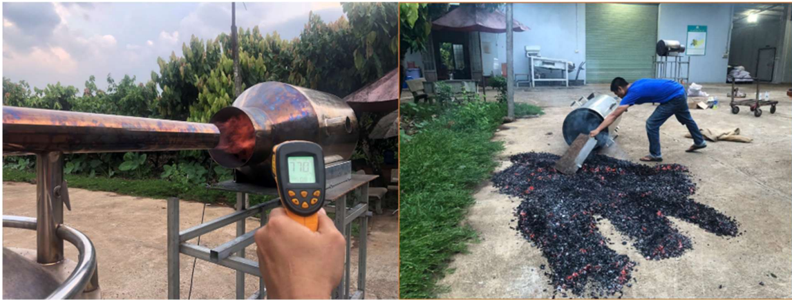
Figure 1: A semi-industrial Torch Updraft Gasifier at Trong Duc Cacao Company
